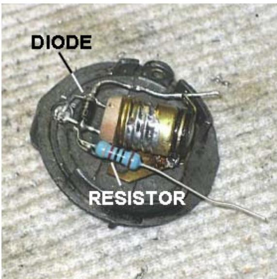
4. Solder a rectifier (1N4001 shown) across the LED leads. The "arrow point" of the rectifier (the lined end) should be connected to the positive LED lead. After soldering, clip the left rectifier lead as shown and solder the resistor (1 K ohm, 1/2 watt shown) to the clipped lead. Bend the other rectifier lead down along the side of the socket parallel to the resistor.
