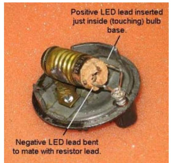
Positive LED lead inserted just inside (touching) bulb base.
