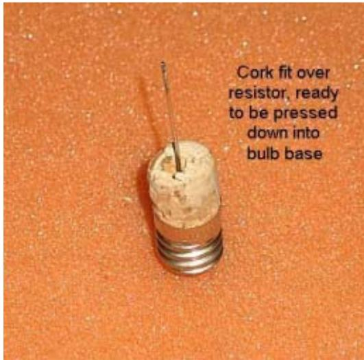
Cork fit over resistor, ready to be pressed down into bulb base
