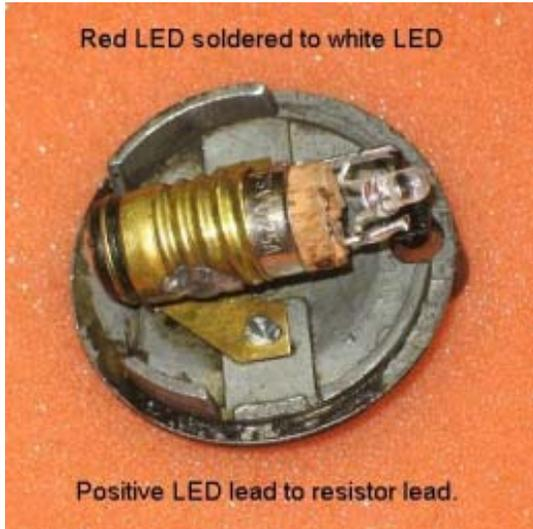
11. Solder the positive lead of the red LED to the resistor lead & negative white LED lead. Solder the negative lead of the red LED to the positive lead of the white LED.
