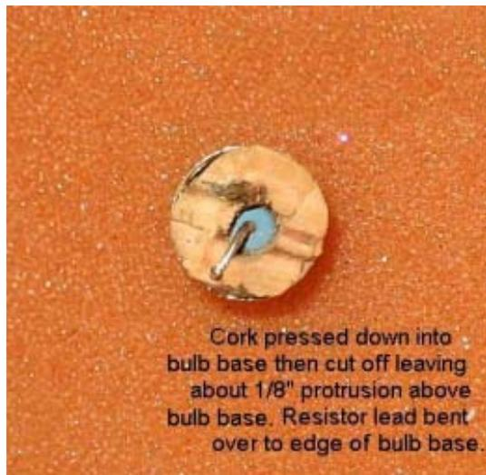
Cork pressed down into bulb base then cut off leaving about 1/8" protrusion above bulb base. Resistor lead bent over to edge of bulb base.
