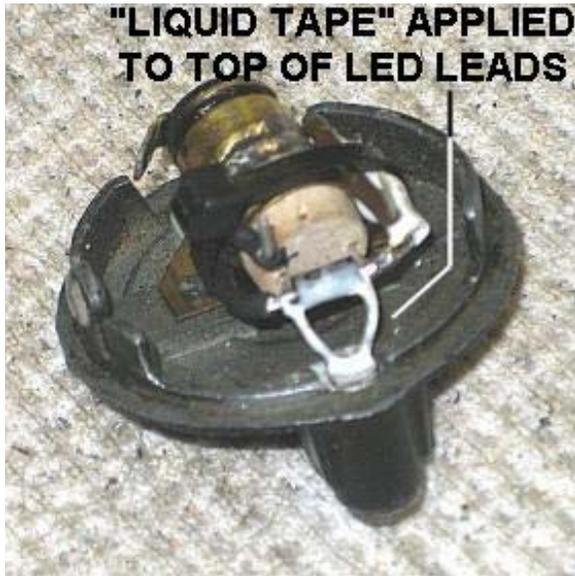
8. Although the "fit" of this assembly checks out OK, a little electrical insurance will be obtained by coating the LED leads with a dab of "liquid tape" as shown. Although white is shown here (it was handy), black is also available. Black may be preferable ... if it is also used to also coat the back of the LED, it will help prevent any light leaks around the edge of the boiler front if it does not seal tightly against the boiler shell.
