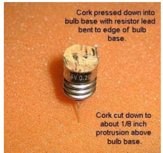
Cork pressed down into bulb base with resistor lead bent to edge of bulb base.
