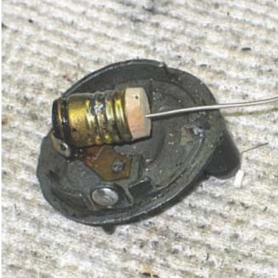
2. Using a small diameter probe (20 gauge copper wire with insulation stripped shown here), poke two holes in the cork near the outer edges, on a diameter parallel to the boiler front. The holes need to be far enough apart for the rectifier to fit between them. Be careful that the holes do not allow contact with the socket sides as these holes will be the mounting holes for the LED leads.
