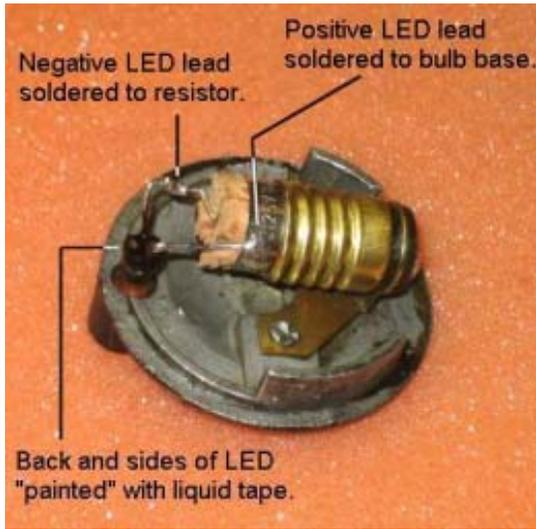
9. Solder the positive LED lead to the bulb base and the negative LED lead to the resistor lead. Optional – coat the sides and back of the LED with black “Liquid Tape” (or black paint). This will help prevent any white light leaks around the boiler front if it does not seal tightly against the boiler shell.
