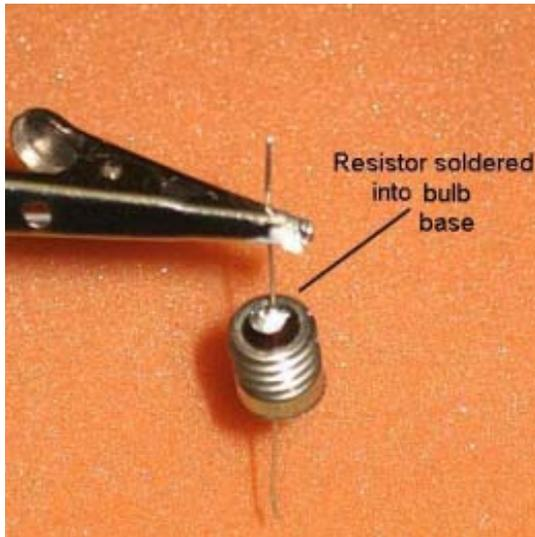
4. Solder the resistor lead to the center contact of the bulb base as shown.
