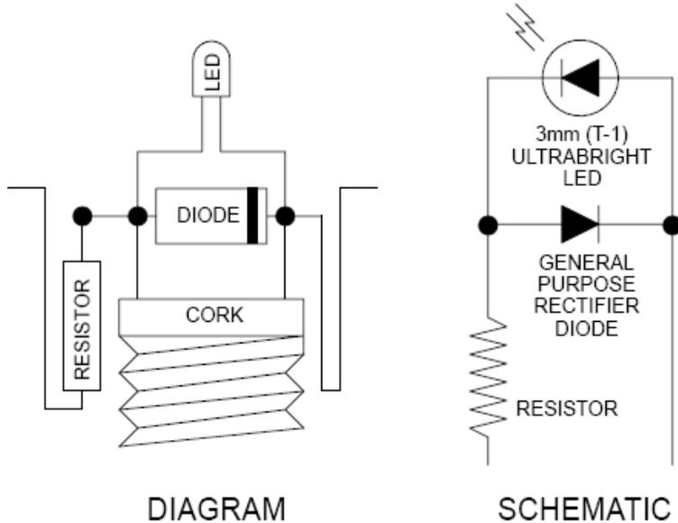
The figures to the left provide a simplified diagram of the component layout, and an electrical schematic. What follows is a pictorial presentation on assembling the components. A limited discussion of electrical considerations is at the end of this document.
