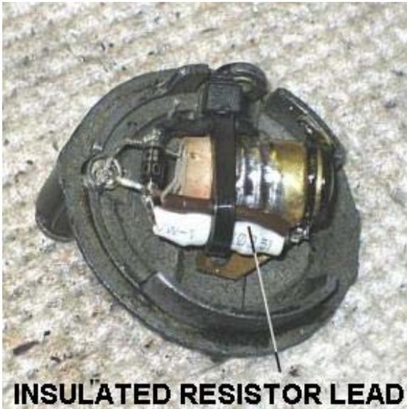
6. Bend the insulated rectifier and resistor leads back up toward the top of the boiler front (essentially bending them back on themselves), and secure them in position with a small tie wrap around the socket. As the leads are insulated and the socket will not be energized, a wire tie could also be used to hold these components together. This rigidity is required to insure that the electrical connection points cannot move around within the boiler.
