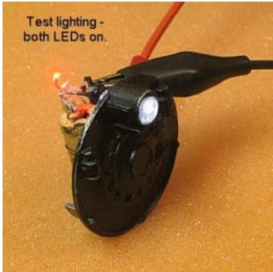
13. Test power the finished assembly – both LEDs should be illuminated.
